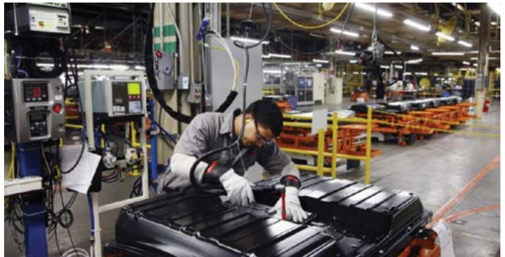
Bottom: An employee at the Nissan plant in Smyrna, Tennessee finalizes the fabrication of a lithium-ion cell battery pack assembly. CIS partners with Nissan to provide Nissan-specific supplier development training to their supplier network.
